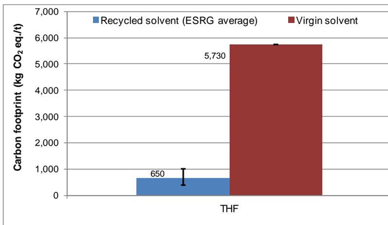
**Figure 6-4 Comparison of recycled THF with the virgin solvent**
