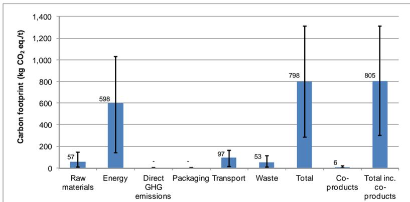
**Figure 7-2 Carbon footprint of 1,000 kg of recycled MEK by data category**
