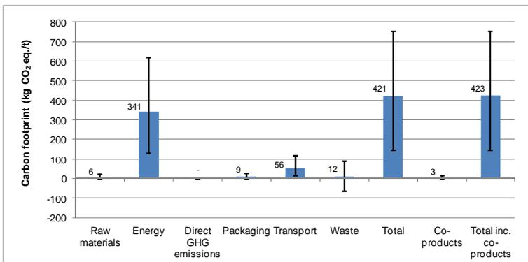
**Figure 5-2 Carbon footprint of 1,000 kg of recycled acetone by data category**
