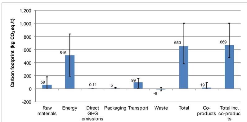
**Figure 6-2 Carbon footprint of 1,000 kg of recycled THF by data category**
